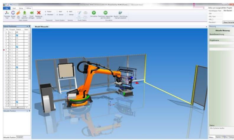
Certain automation software solutions have a completely modular outlay, providing open interfaces in every direction. Various robot types, sensors as well as evaluation software packages can be connected with each other, hence offering flexibility and independence. An integrated collision control during offline programming increases the operational safety and reduces the overall system occupancy time.
