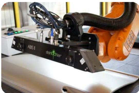
Due to the permanently increasing competition and cost pressure an early and objective detection of surface imperfections during the production process is indispensable. The corresponding tool and production processes can be immediately optimized with the result, which in turn increases the efficiency of the quality control. This also has a positive reaction on the improvement of the surface as well as the economic application of working hours and raw materials.
